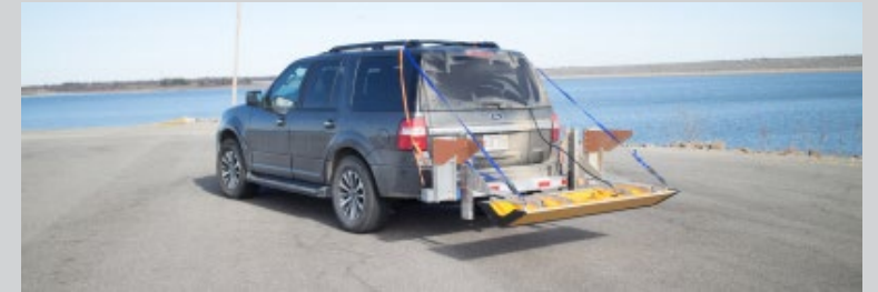
Air-Launched 3D GPR | Source: Infrasense
