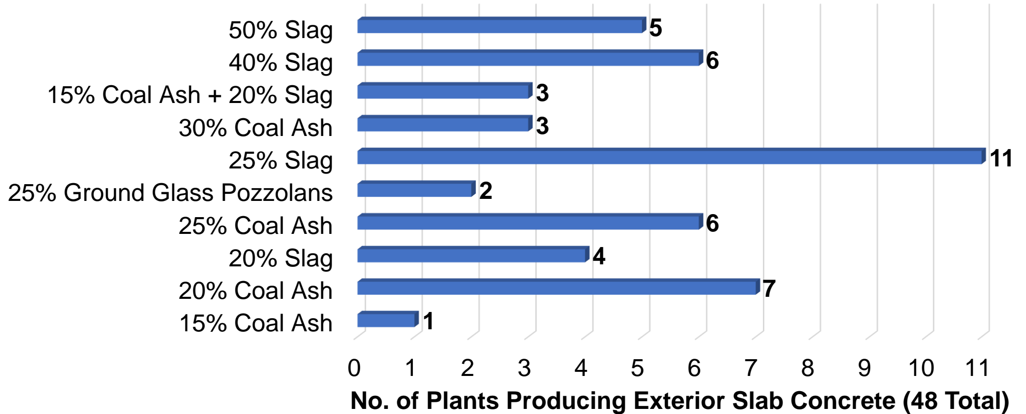
Plant Distribution of Exterior Slab Concrete Mix Designs
