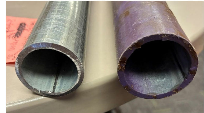
Zinc Galvanized Tubes w/out epoxy with A934 epoxy
