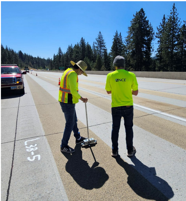
Face Dipstick Profiler – Transverse Profile Measurements
