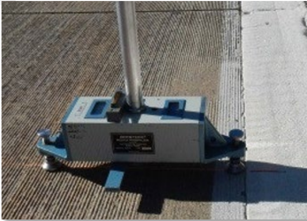
Face Dipstick Profiler – Transverse Profile Measurements
