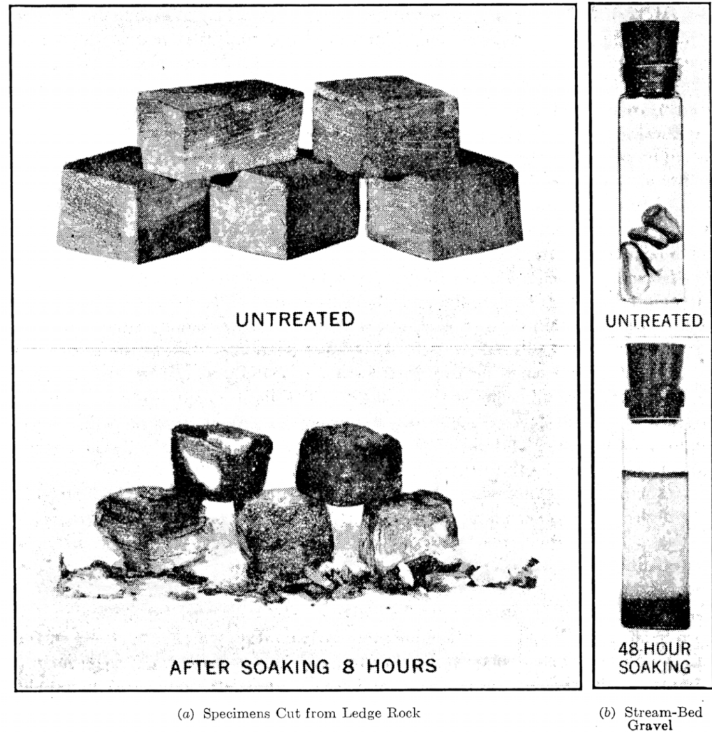
FIG. 9.—EFFECT OF A 10% SODIUM HYDROXIDE SOLUTION (AT 70° F) ON SOME TYPES OF SILICEOUS (CHERTY) SHALE AND CHERT FROM THE CALIFORNIA MIOCENE FORMATIONS
