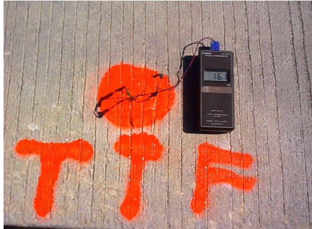
Maturity probe location with hand held thermometer
