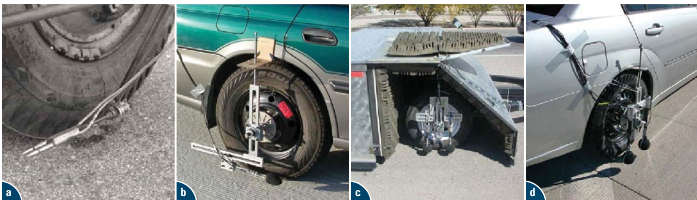
Figure 5. Development of the OBSI test fixture over time
