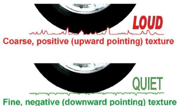
Figure 3. Idealized texture for loud and quiet pavements
