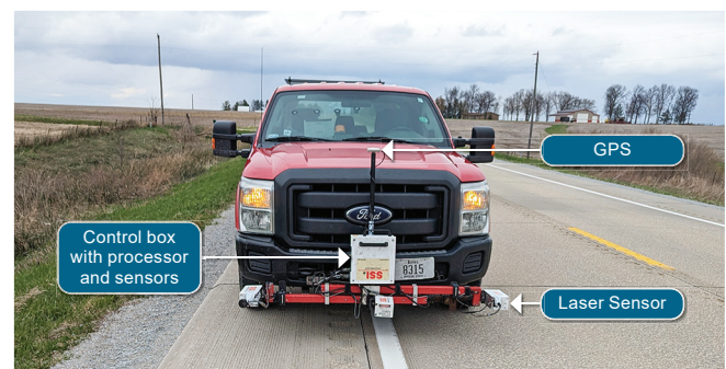
High-speed surface profiling system for pavement smoothness and curling/warping measurements
