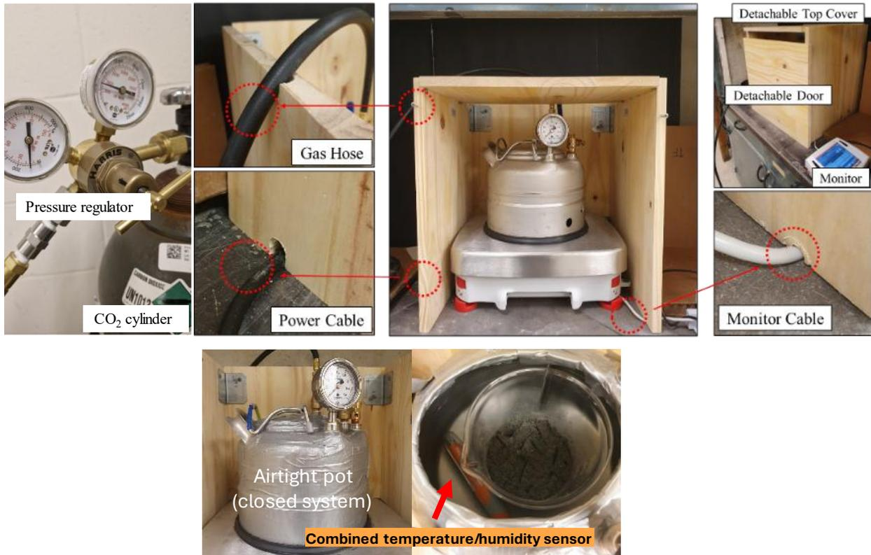
**Figure 4.1. Experimental setup for the carbon treatment**
