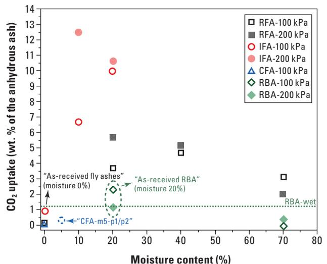
Effect of ash moisture content on carbon intake
