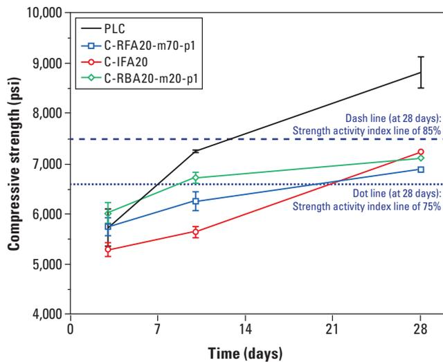
*Compressive strength of mortar cubes containing carbon-treated ashes and subjected to carbon curing after casting*
