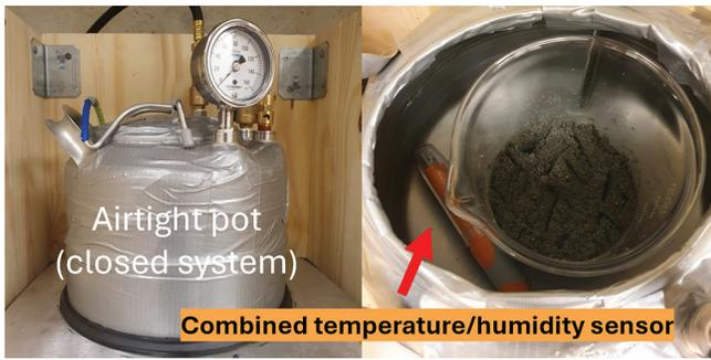
Experimental setup for carbon treatment: carbon chamber (left) and sample in the chamber (right)
