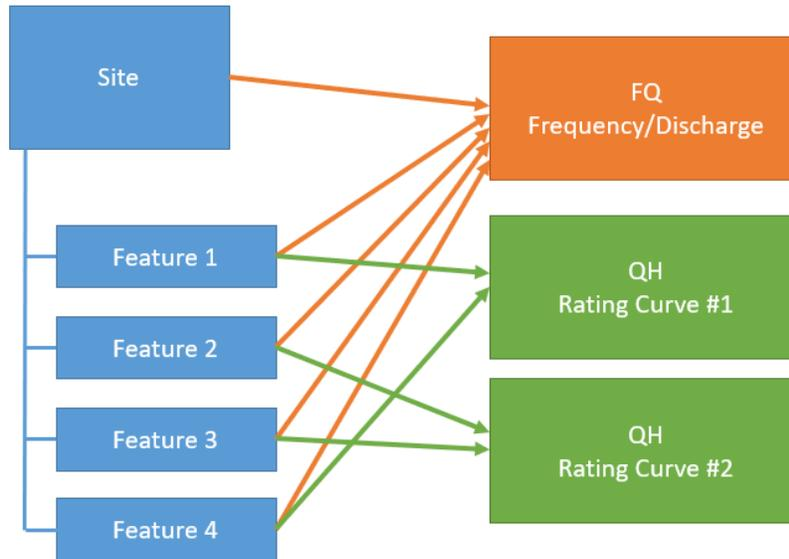
**Figure 2. Overview of site/features and hydraulic components**
