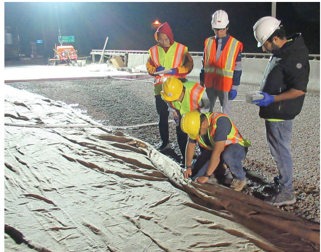
SR measurement performed on field overlay three hours after casting
