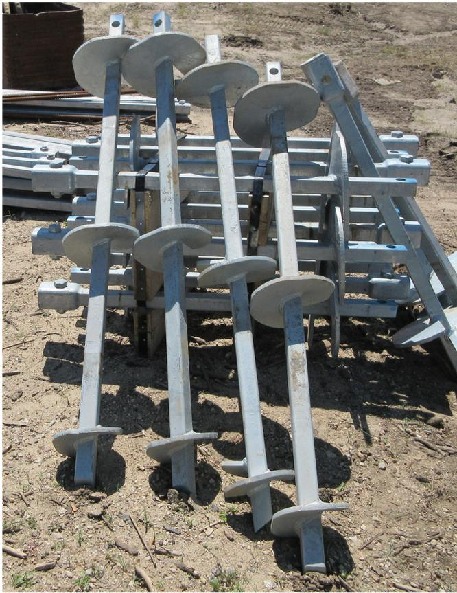
*Helical pile lead sections*
