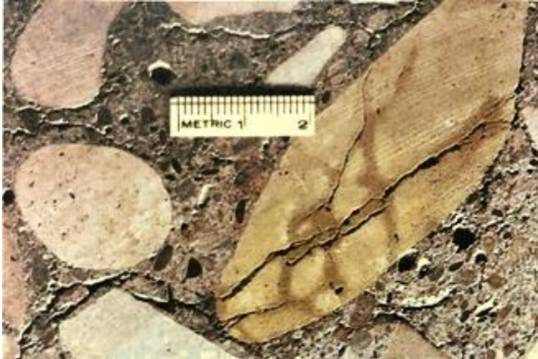
Figure 3. Cracks propagate within the coarse aggregate structure
