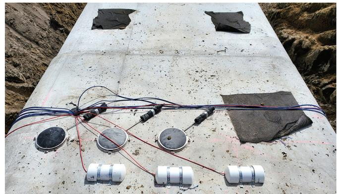
*Crawford County pressure cells and strain gauges for one of three culvert sections*
