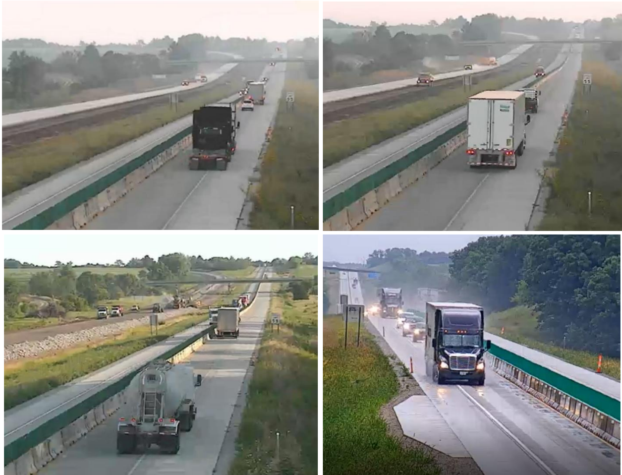
Figure 13. Examples of trucks positioned well over right lane line in the presence of PCBs
