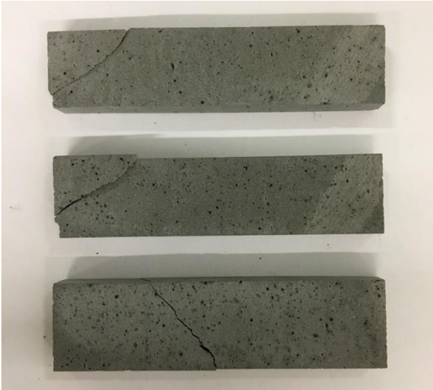
Figure 6.4. Failures during direct tension tests
