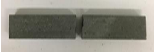
(b) Sample loaded perpendicular to printed filaments
