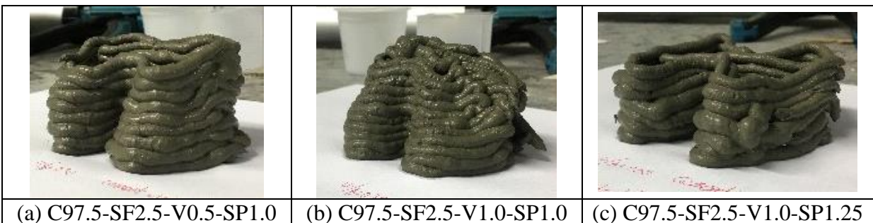
Figure 3.4. Effects of chemical admixtures on the printing qualities of mixtures with silica fume
