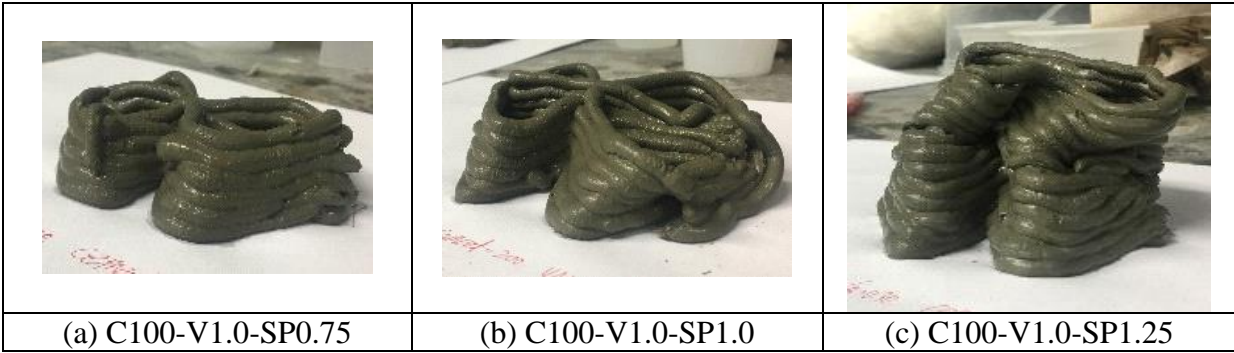
Figure 3.3. Effects of superplasticizer on the 3D printing by syringe
