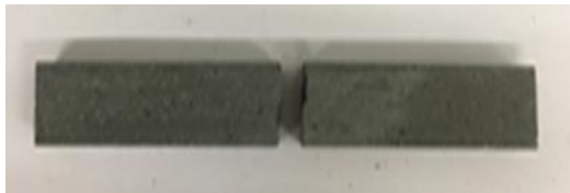
(c) Sample loaded parallel to printed filaments
