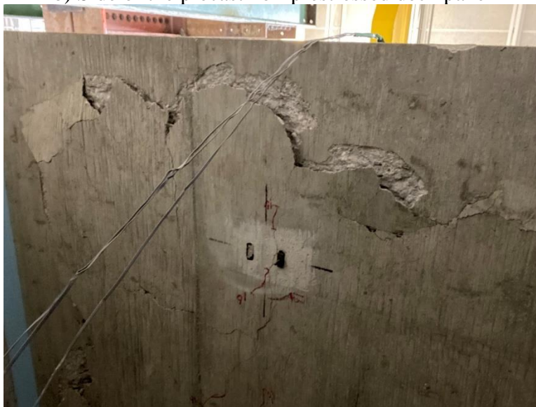
c) Spalling of deck concrete at the bottom of the deck
