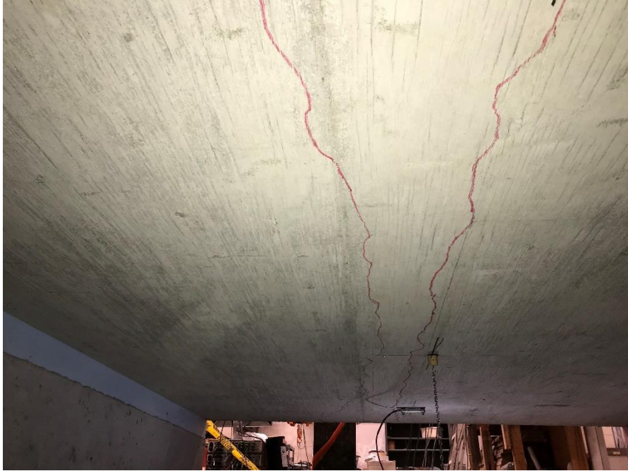
Figure 33. Crack on the bottom surface of deck after LC6
