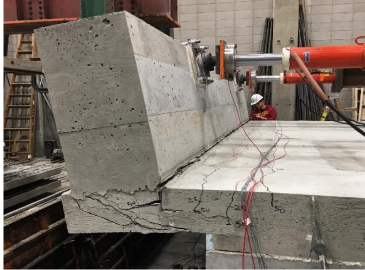
Figure 26. Precast deck concrete crash (Specimen I)
