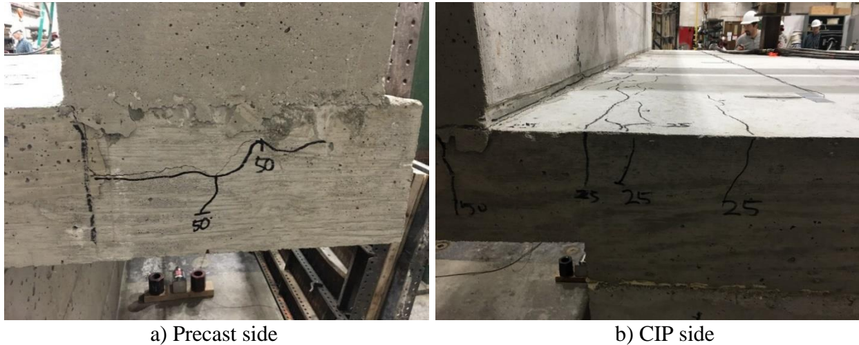
Figure 25. Cracks under the barrier (Specimen I)
