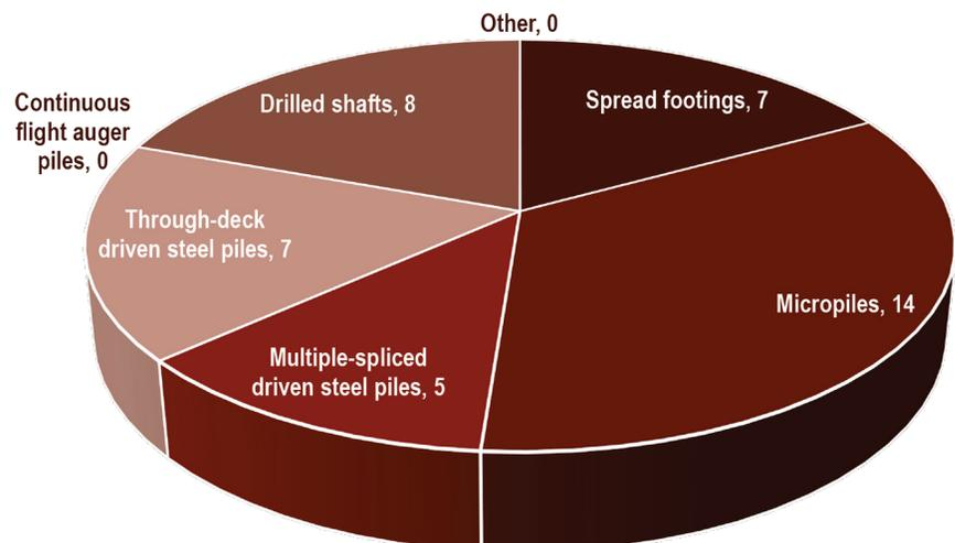
Survey results for types of solutions agencies use when constructing a new foundation beneath an existing bridge
