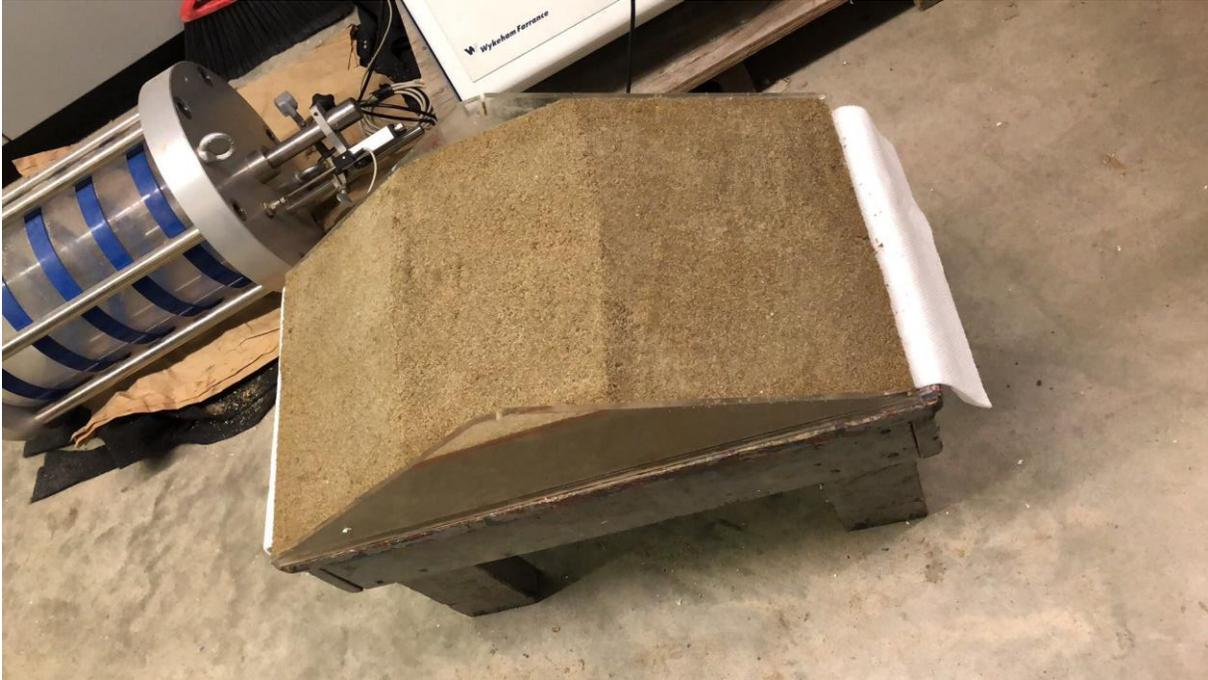
**Figure 4. Levee model before testing**
