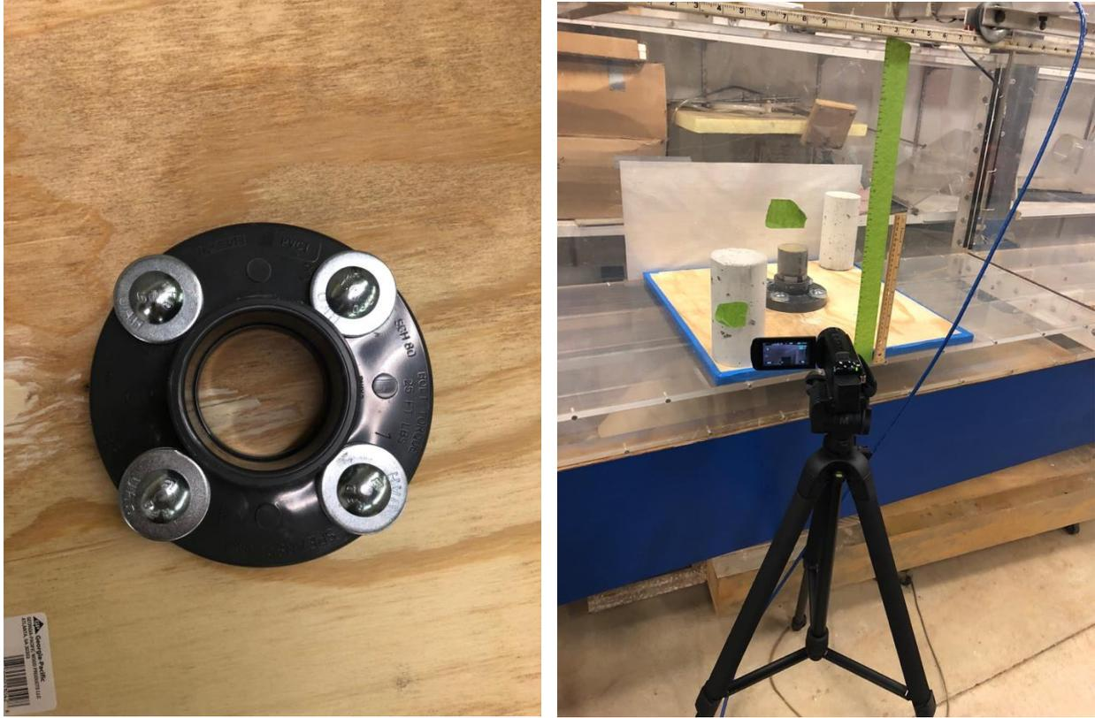
**Figure 2. Flange attached on the plywood (left) and flume test set up (right)**
