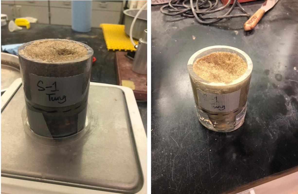
**Figure 7. MICP treated specimen after flume test (left) and untreated specimen after flume test (right)**
