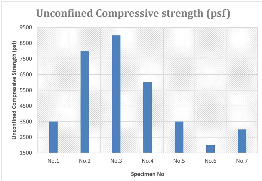
**Figure 9. Unconfined compressive strength of controlled specimens**
