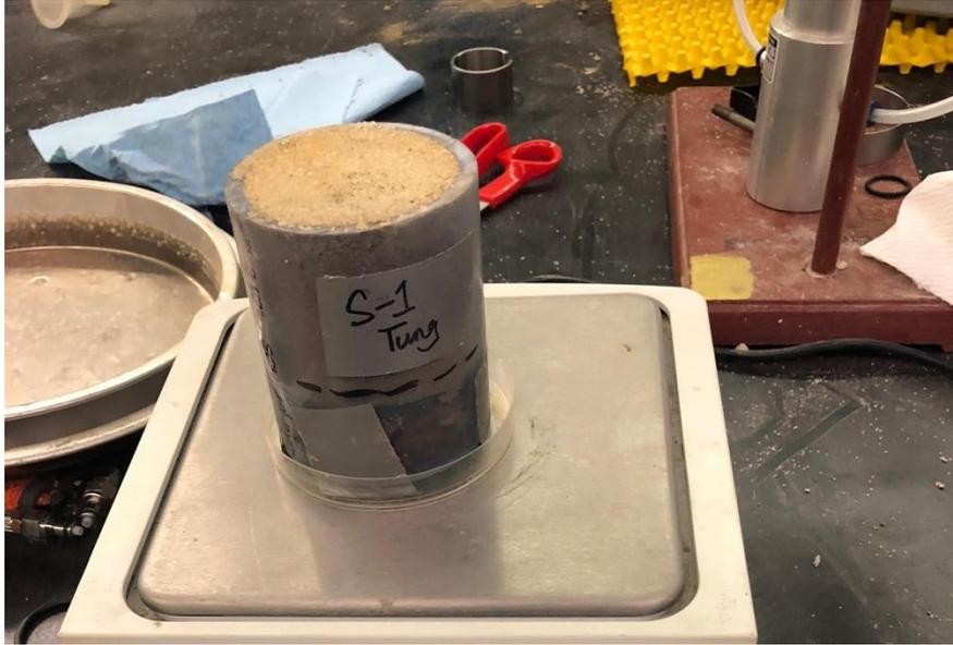
**Figure 1. Typical soil column specimen**
