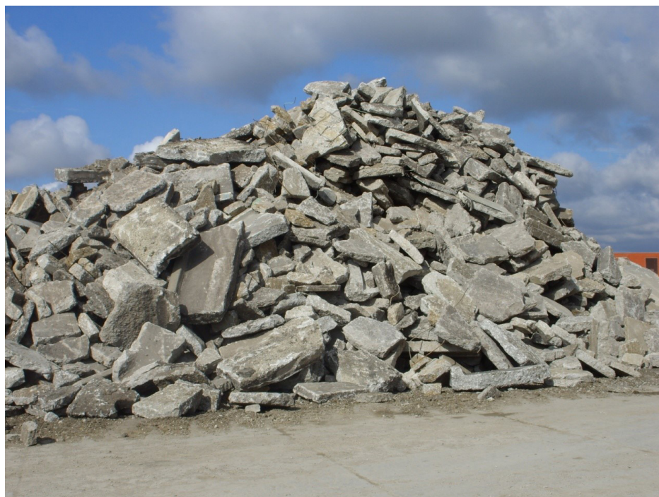
Figure 1. Stockpile of broken concrete to be recycled (Photo courtesy of Jerod Gross, Snyder & Associates, Inc.)
