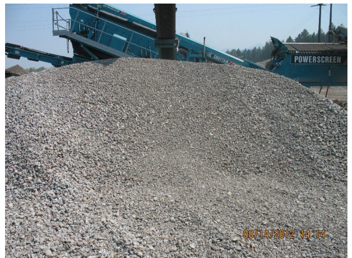
Figure 6. RCA produced for North Park Road Project (Photo courtesy of Phillip Lamoureux, FHWA WFL)
