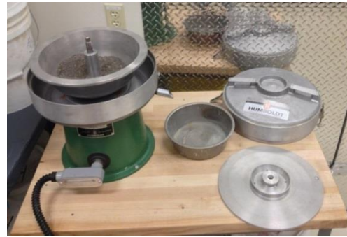
Figure 4. Illustration of the centrifuge, which has been used to determine the moisture properties of lightweight fine aggregate
