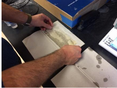
Figure 1—Tapping of the wet teabag during the absorption calculation process
