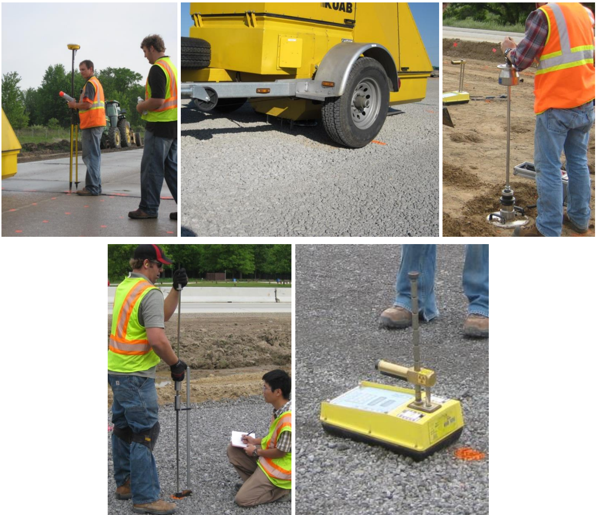
Figure 1. Trimble SPS-881 hand-held receiver, Kuab falling weight deflectometer, and Zorn light weight deflectometer (top left to right); dynamic cone penetrometer, nuclear gauge, and nuclear gauge (bottom left to right)
