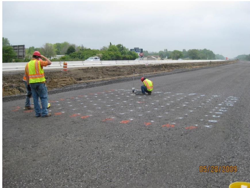
Figure 8. MI I-94 TS1b: Photograph showing testing on the 0.6 m x 0.6 m grid pattern
