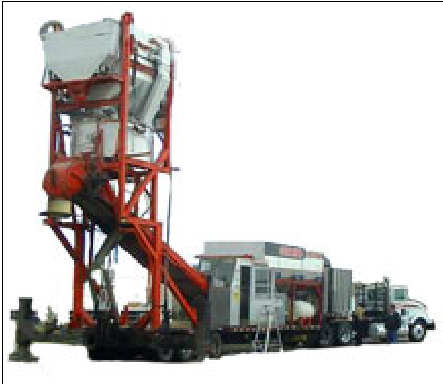
Figure 35. Two-stage mixing plant (Concrete Mobility 2007)
