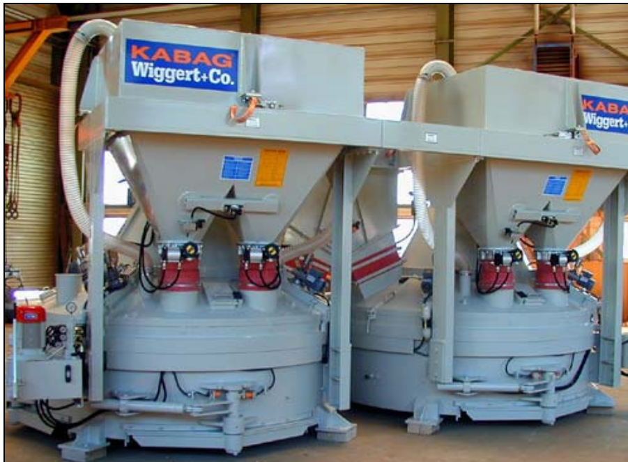
Figure 38. Two countercurrent concrete mixers working in tandem (Advanced Concrete Technologies 2007)
