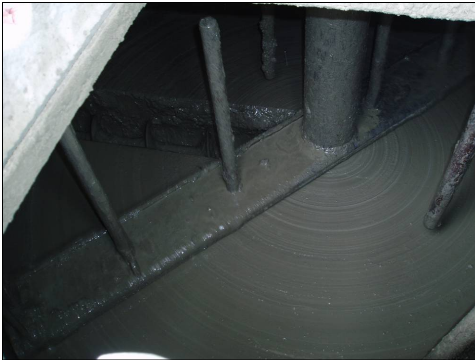
Figure 52. Rotating fingers in the slurry pre-mixer
