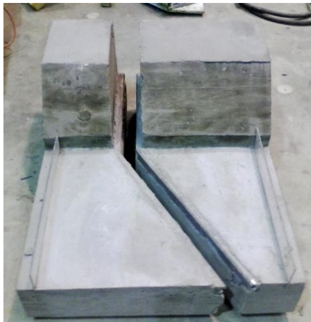
Figure 46. Finished barrier rail for straight-through and dogleg detail
