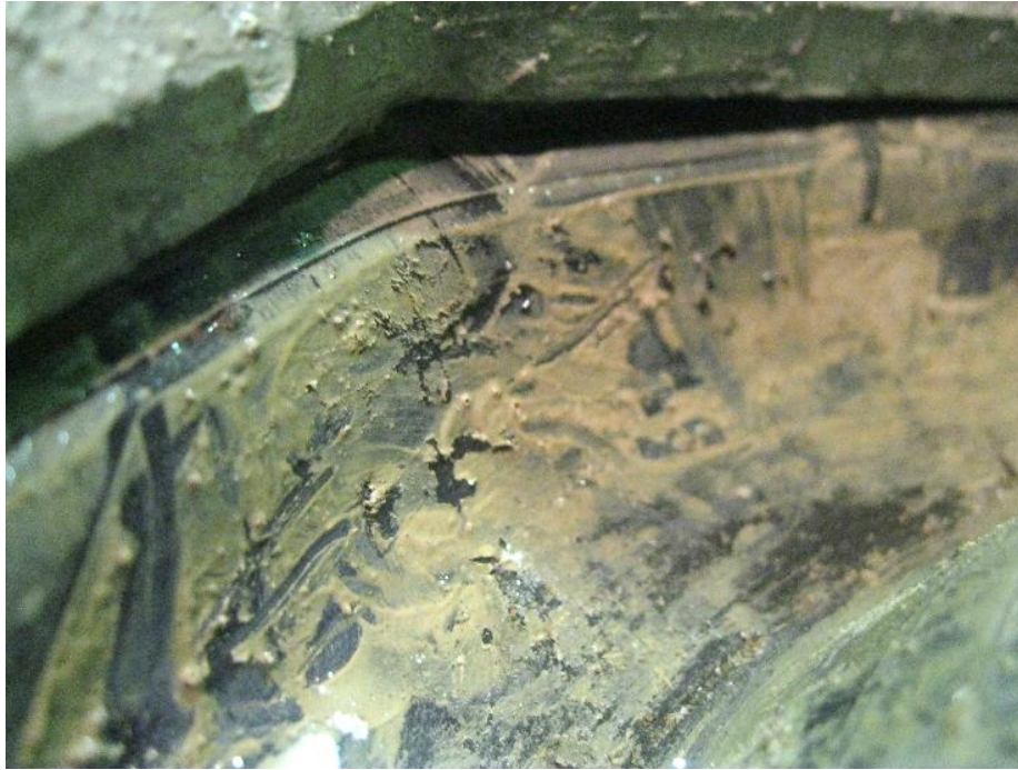
Figure 55. Improper gland installation causing leak in Watson Bowman Acme dogleg specimen
