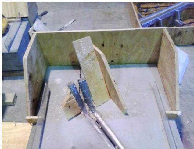
Figure 34. Plywood used to create foam enclosure
