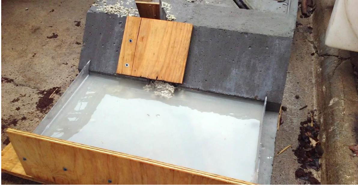
Figure 61. Bentonite option specimen during ponding test
