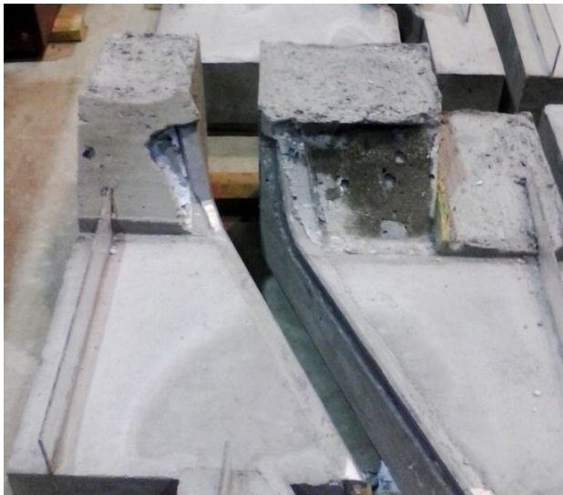
Figure 39. Turn-up portion of the strip seal encapsulated in concrete at the same time the deck was poured
