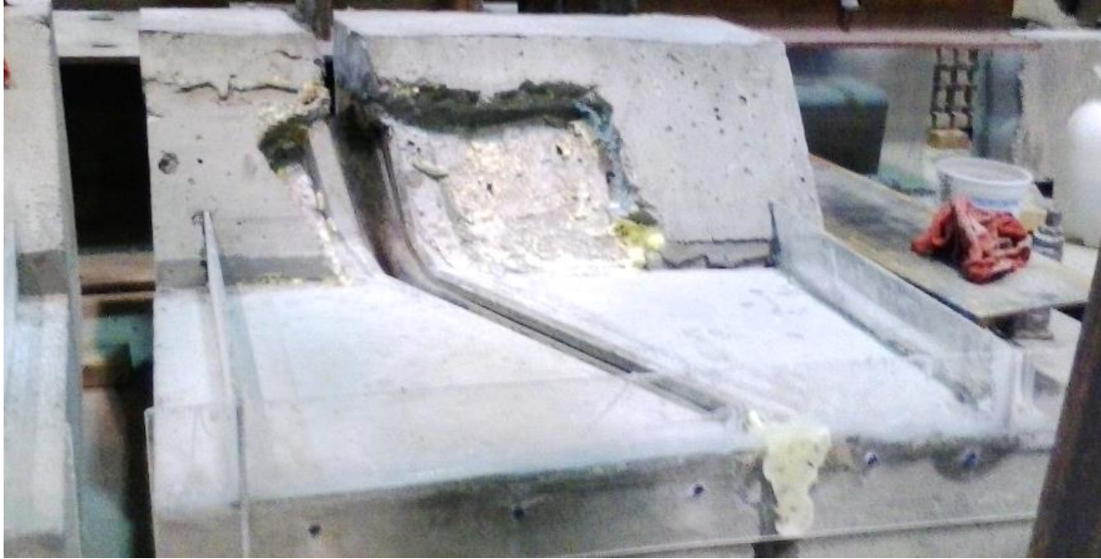
Figure 40. Completed barrier rail
