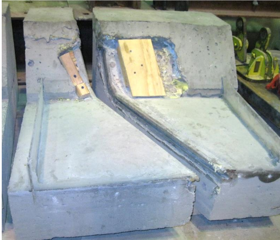
Figure 42. Wood attached in the blackout area to reduce the size of the working room, only leaving room directly in front of the extrusions
