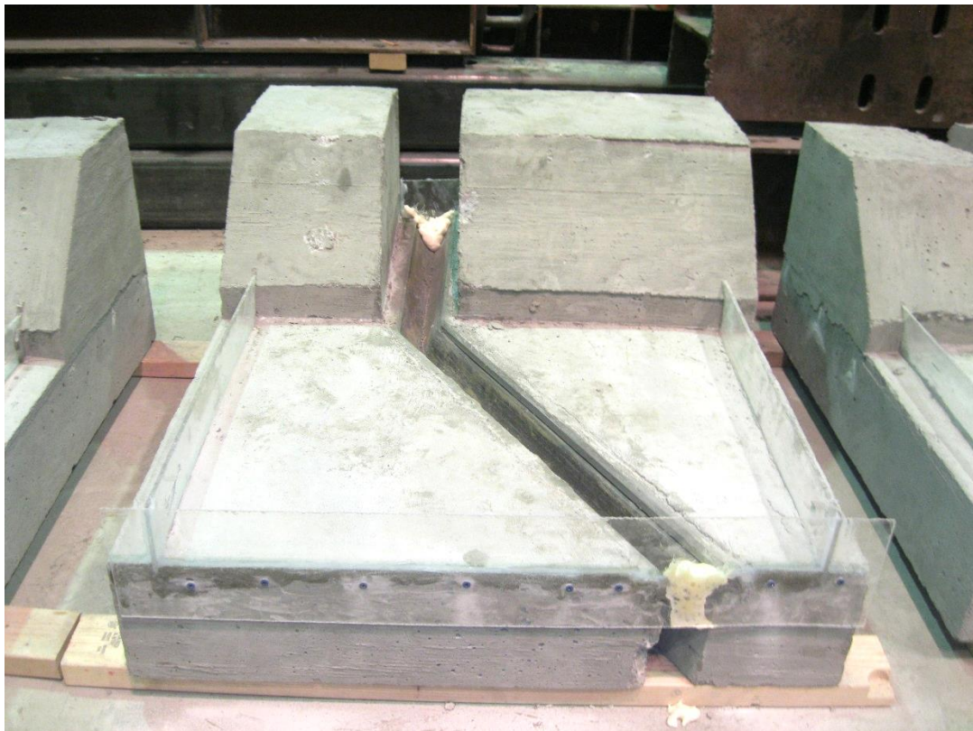
Figure 49. Straight-through dogleg termination specimen using Watson Bowman Acme seal
