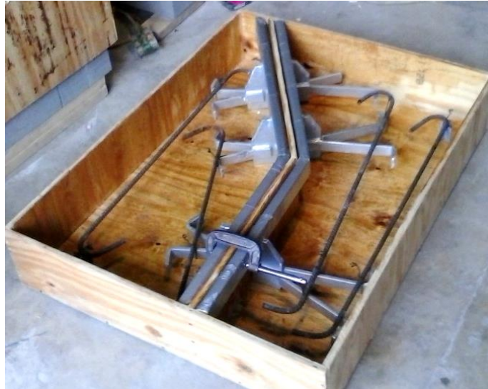
Figure 43. Deck formwork for straight-through and dogleg specimens
