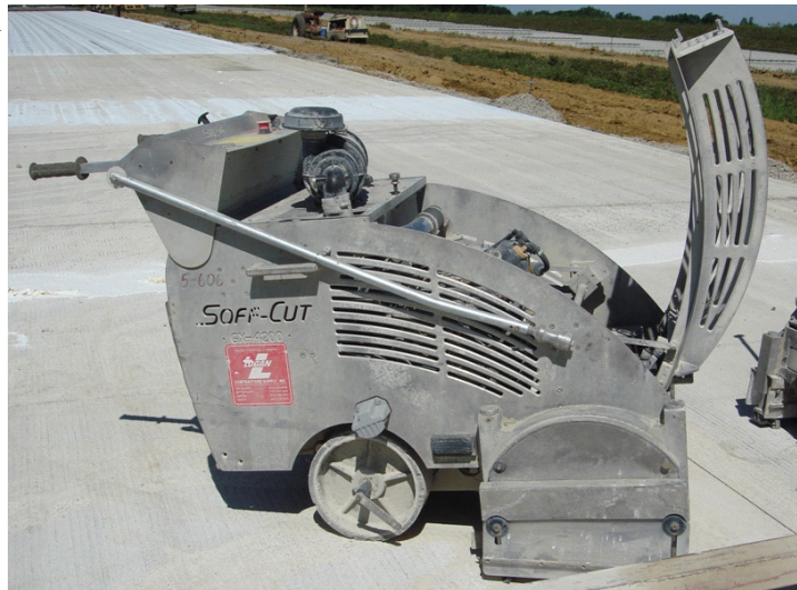
(a) Early entry sawing
