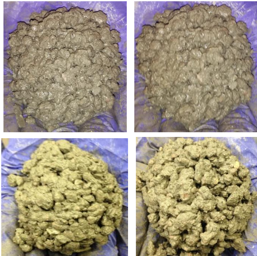
Figure 7. Workability test results of pervious concrete mixtures: Portland cement (top left), Portland cement - 15% Fly ash (top right), Portland cement - 15% Slag (bottom left), and Portland cement - 15% Limestone (bottom right)
