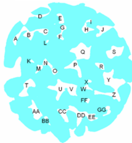
Figure A.9. Pore spaces on each PCPC sample central cross-section, numbered alphabetically
