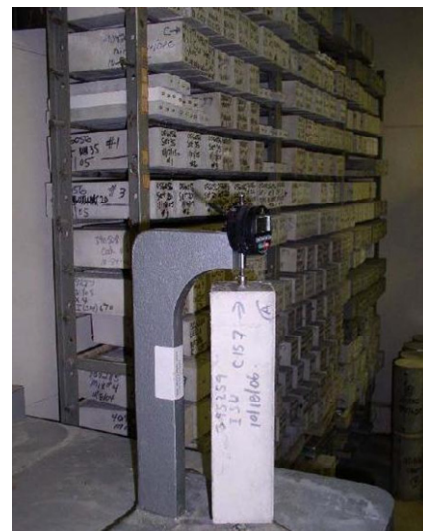
(b) Length comparator and storage area in Environmental room
