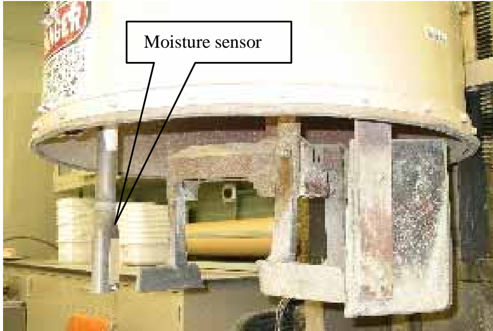
Figure 11. The moisture sensor that was used in this study
