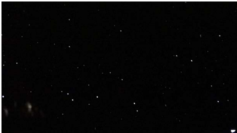
Figure 4.8. Sample of enhanced image of snowflakes obtained using the EDPIV software
