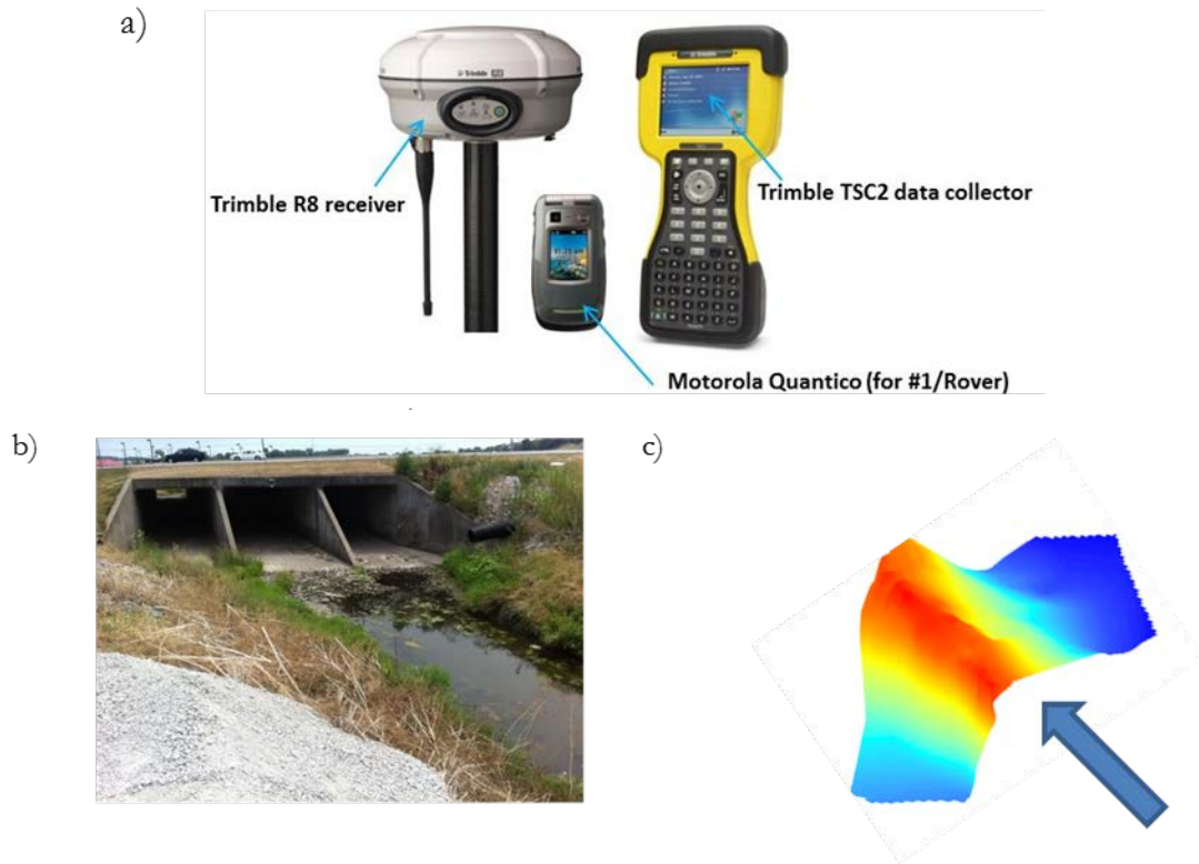
Figure 3.12. Real-time kinematics: (a) components, (b) testing location, (c) mapping result showing bathymetry
