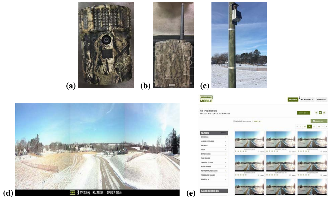
Figure 3.13. Imaging instruments: (a) Moultrie P-180i camera, (b) Moultrie Mobile Field Modem MV1, (c) site with the Moultrie products installed, (d) user interface of the real-time monitoring system, (e) sample image taken from Moultrie camera
