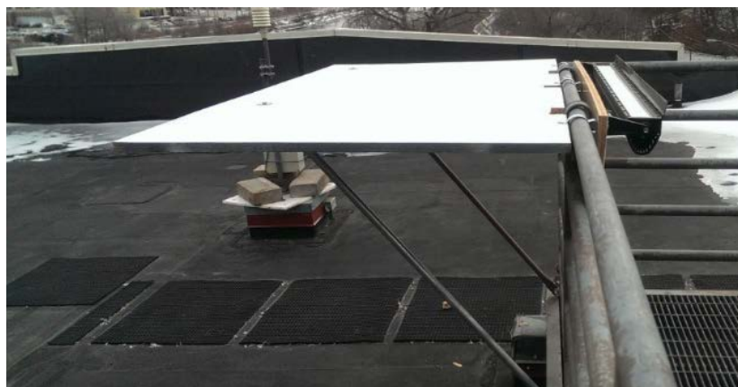
Figure 4.4. Snow measurement board used to measure snow accumulation as part of the rooftop experiment
