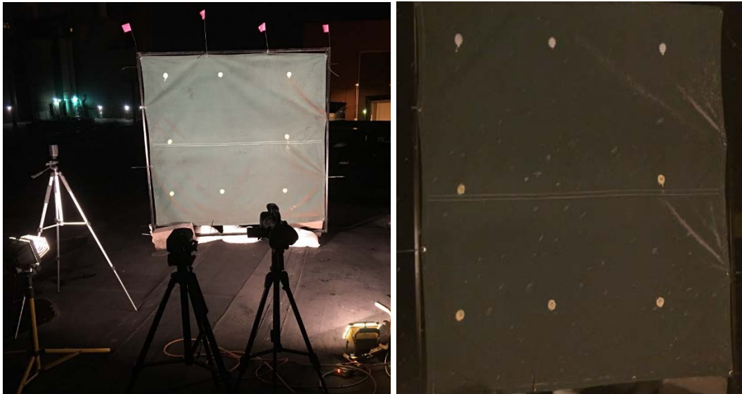
Figure 3.19. Preliminary LSPIV testing: (a) experimental setup and (b) image taken during November 20, 2015 event
