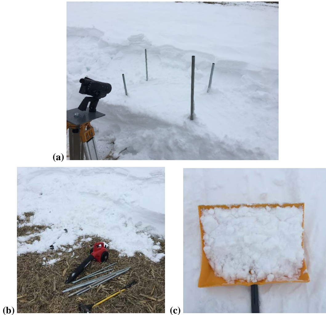
Figure 4.23. Attempt to measure snow drift in situ: (a) test section, (b) snow blower used for entraining the snow, (c) aggregation of snowflakes due to compactness in the snow layer and high temperatures
