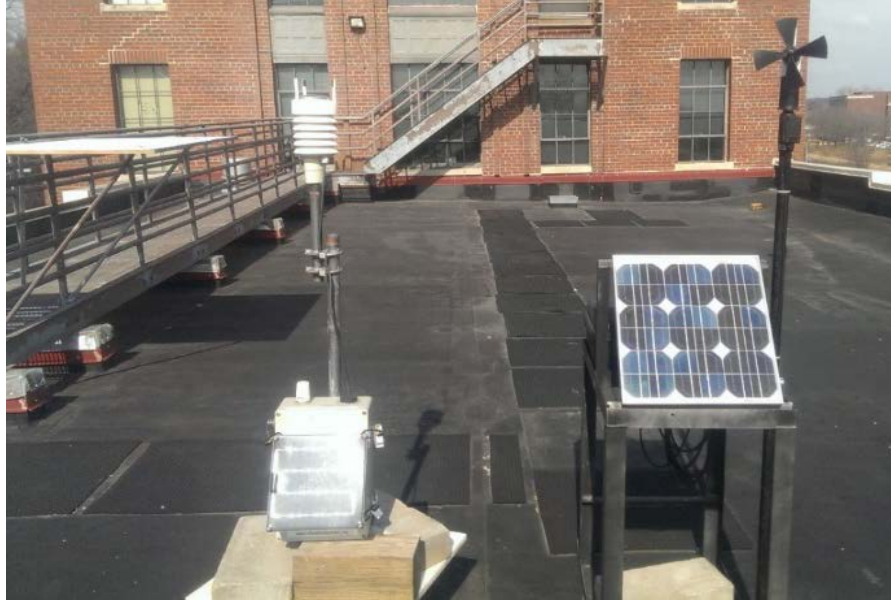
Figure 4.11. Setting of the Vaisala and Young anemometers on the roof of IIHR – Hydrosience & Engineering building
