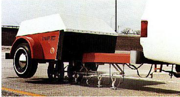
Figure 2.9. Dynaflect (Geo-Log, Inc. 2001)
