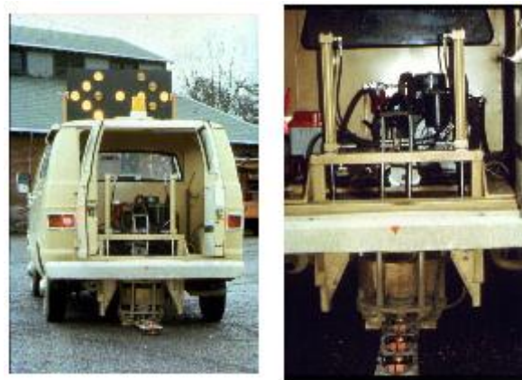
Figure 2.10. Road Rater (Muench et. al., 2005)
