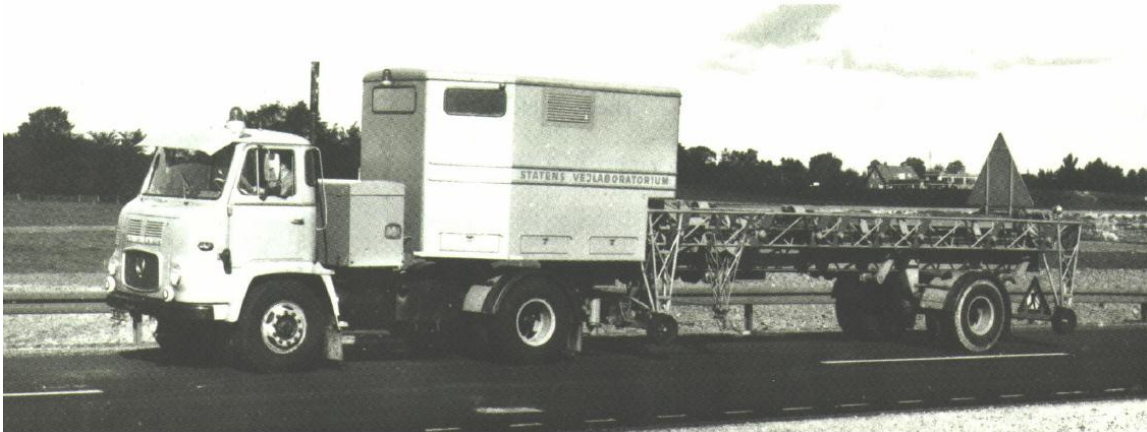
Figure 2.4. The Danish first generation Deflectograph (Christensen, 2003)
