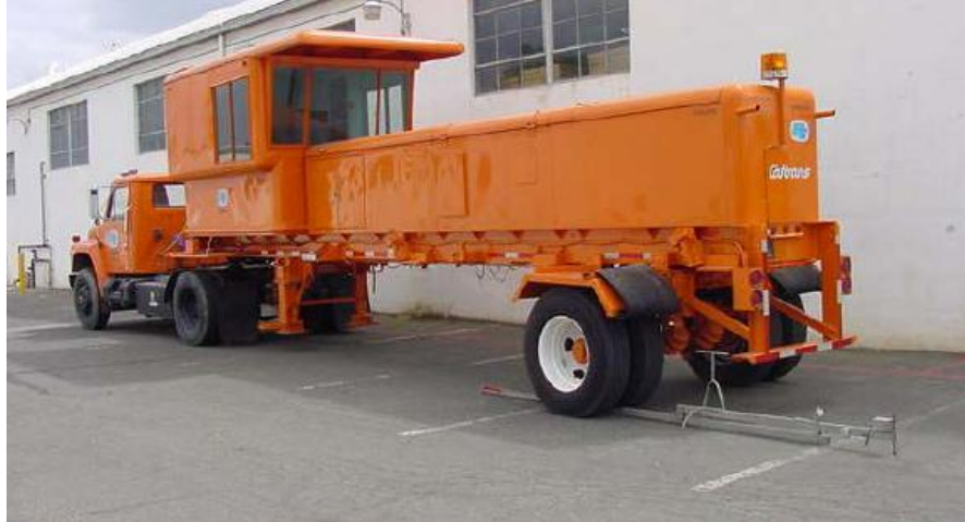
Figure 2.3. California traveling Deflectometer (Andren, 2006)
