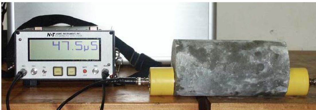
Figure 2.17. Typical ultrasonic test procedure (Ferraro 2003)
