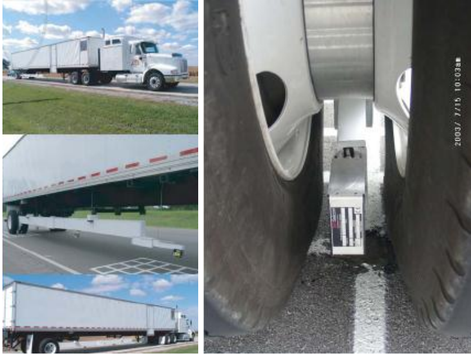
Figure 2.15. RWD prototype (ARA, 2004)
