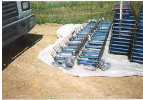
Figure 2. Gage wires connected to frame
