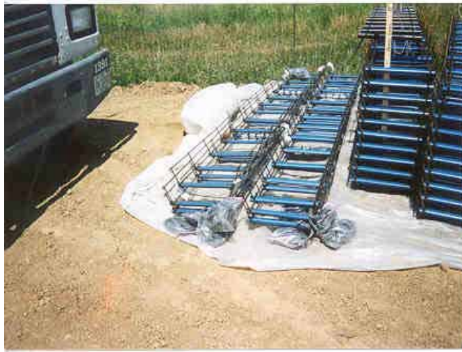
Figure B.1 Gauge wires connected to frame
