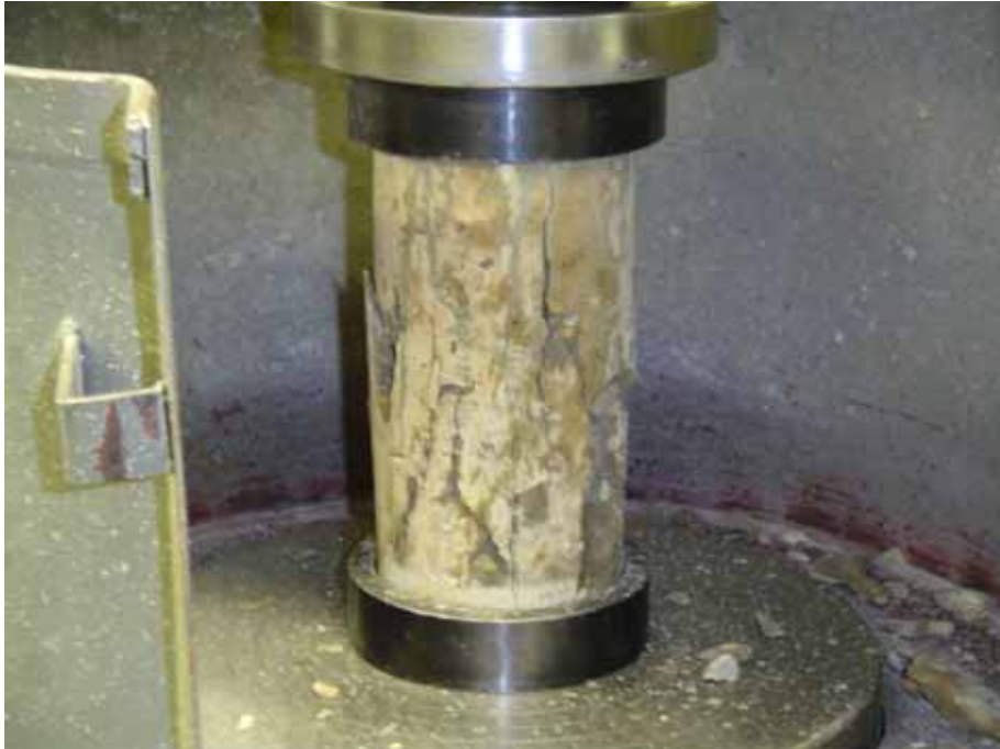
Figure A26. PCC compressive strength test
