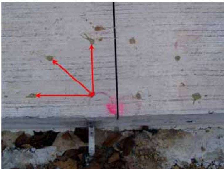
Figure 9. DEMEC points in the “peacock” pattern
