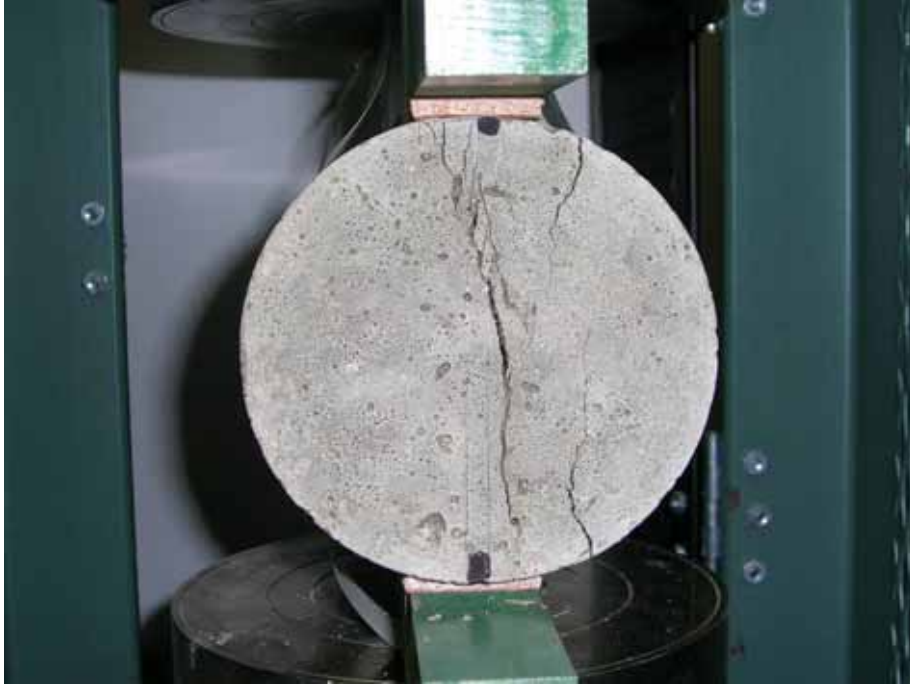
Figure A27. PCC splitting tensile test
