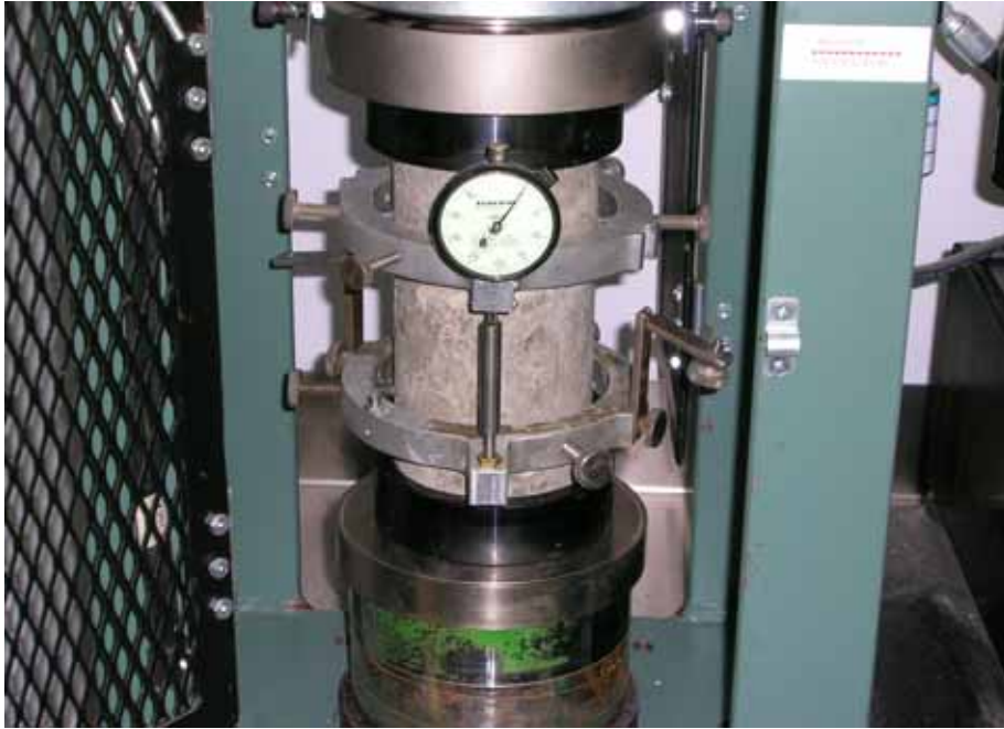
Figure A25. PCC elastic modulus test
