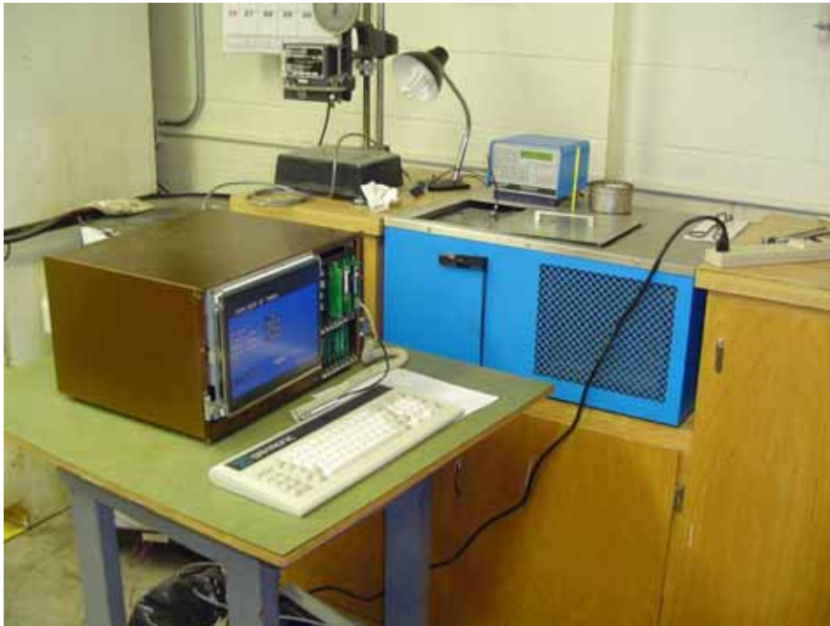
Figure A28. Coefficient of thermal expansion test
