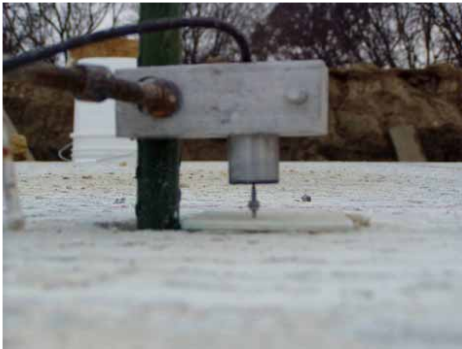
Figure 12. LVDT installation (Iowa State University)
