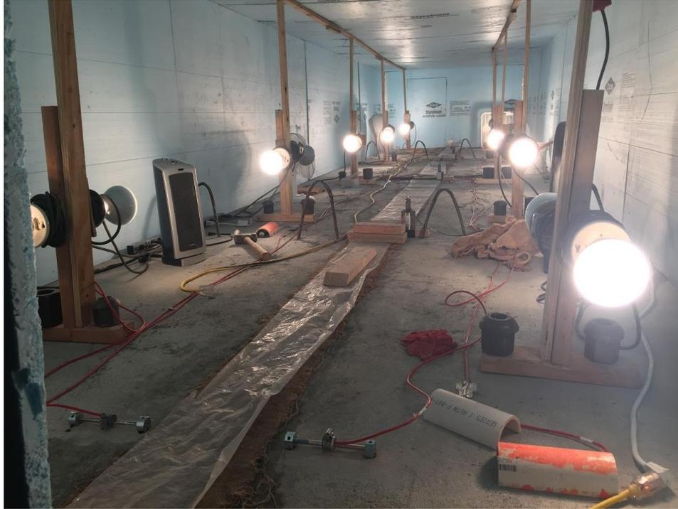
**Figure 27. Heating devices in the temperature isolation room**
