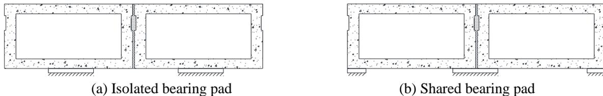
**Figure 6. Common bearing pad details**
