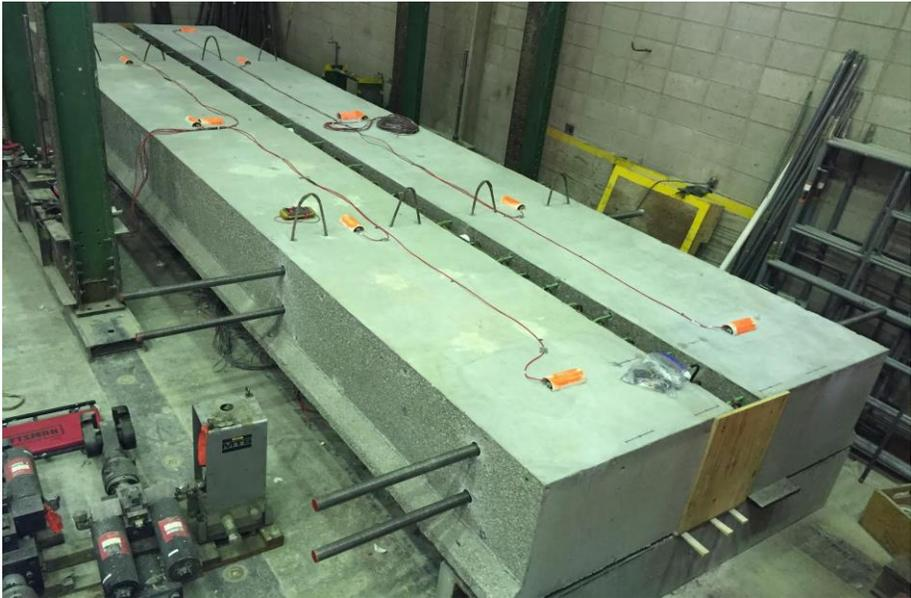
**Figure 25. Specimen before pouring of the joint material**
