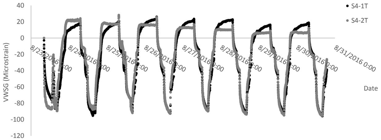
**Figure 76. Strains from Section 4 at the top surface**
