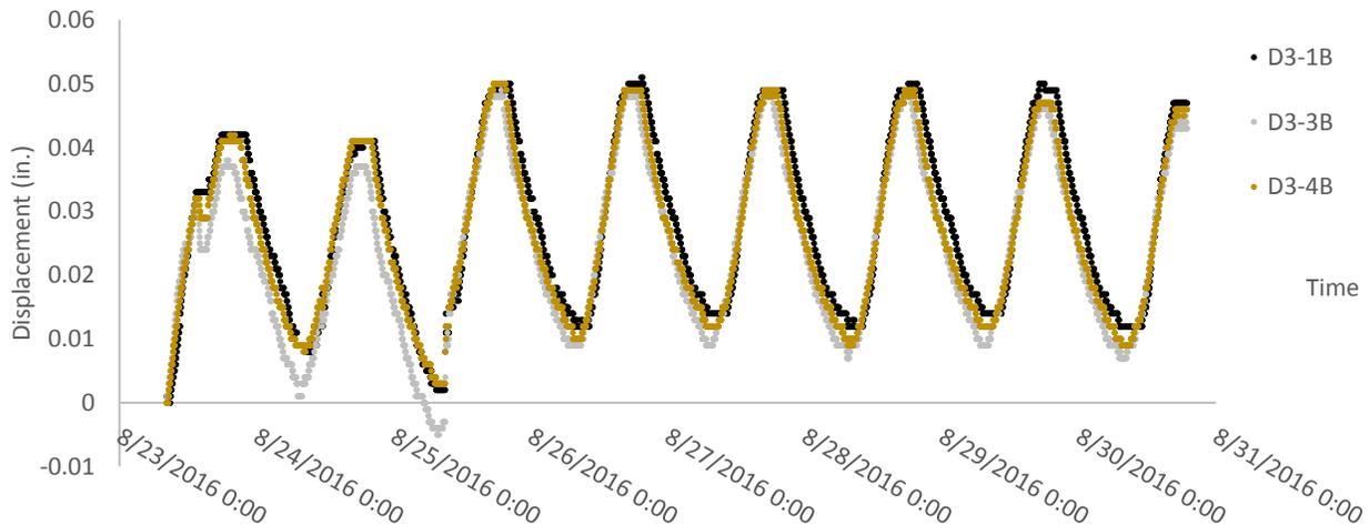
**Figure 79 Vertical displacement at the middle span at early-age**
