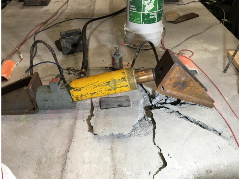
**Figure 94. Crushed box girder due to horizontal load**
