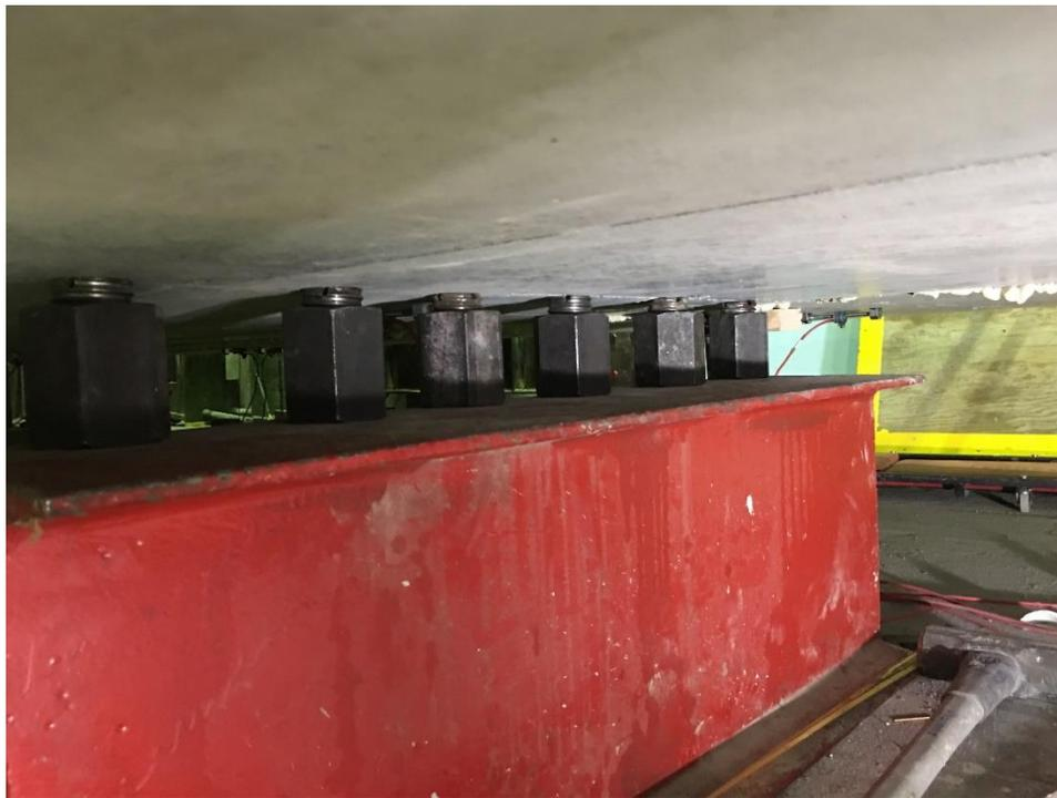
**Figure 36. Restraints under one beam**
