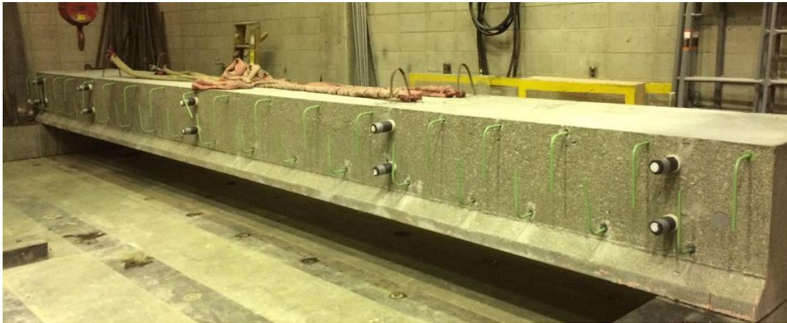
**Figure 23. Side of the box girder with hook bars installed**
