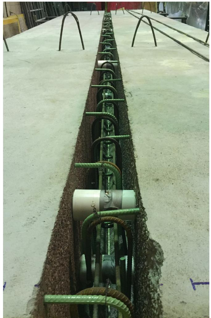
*Two box beams placed side-by-side with roughened interface surfaces for the joint material and reinforcing steel couplers during construction of the innovative wide joint specimen in the laboratory*
