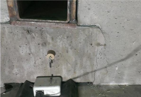
a) Propagation of crack
