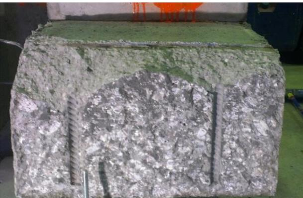
d) Bond interface (overlay concrete)
