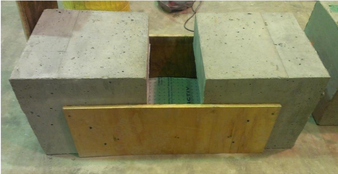
**Figure 29. Push-out test formwork for overlay concrete placement**
