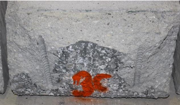
d) Bond interface (overlay concrete)
