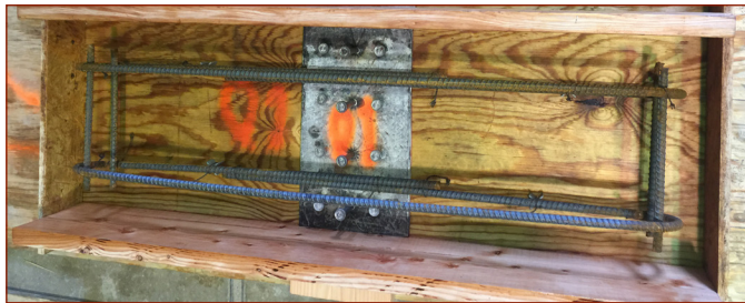
Positive bending flexural test formwork for substrate concrete with steel plate under the reinforcing steel bars
