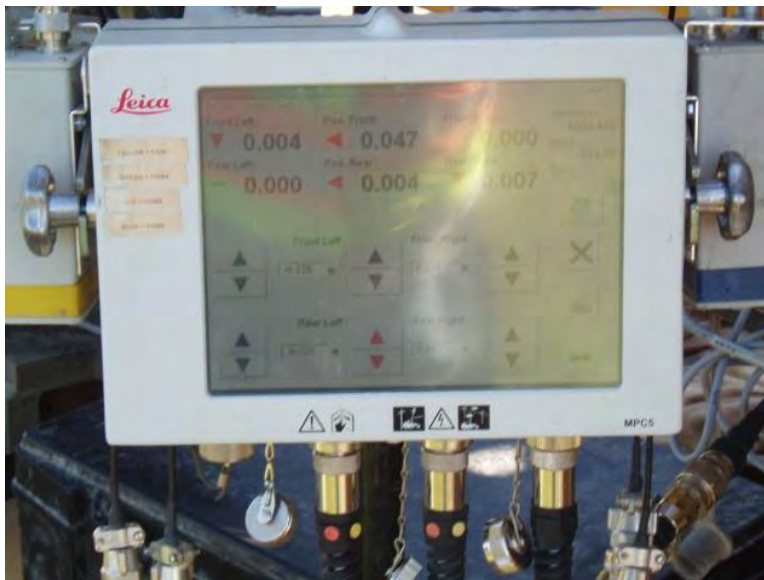
Figure 75. Stringless paver controller
