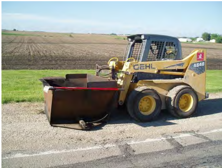
Figure 34. Longitudinal patch filling device
