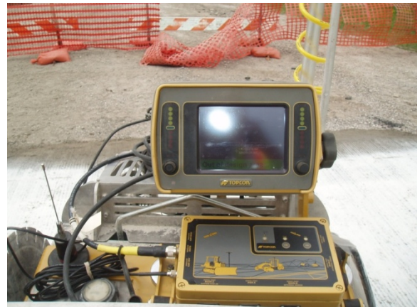
Figures 4 & 5. Standard Concrete Saw Outfitted with GPS Unit
