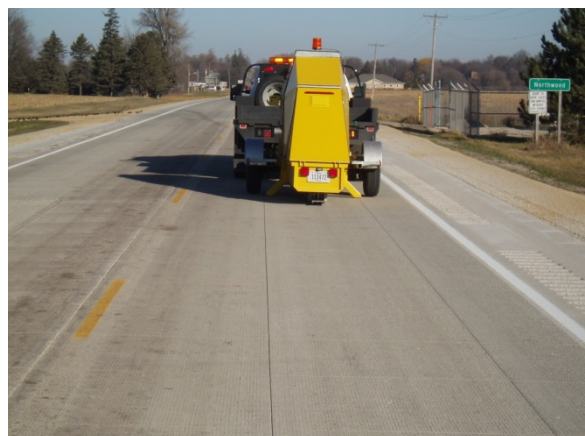
Figures 15 & 16. Falling Weight Deflectometer Testing
