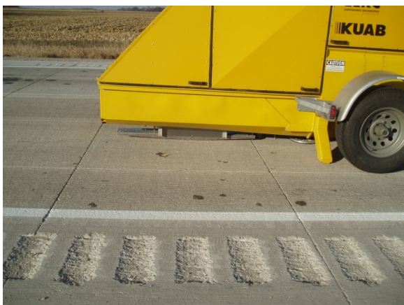
Figures 15 & 16. Falling Weight Deflectometer Testing
