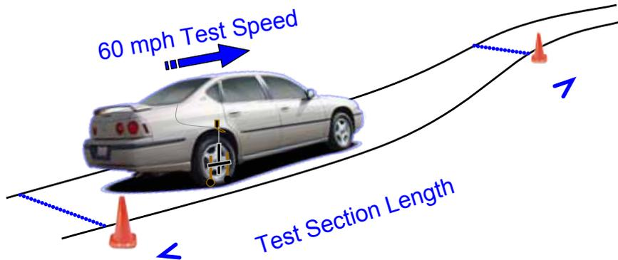
Figure 2. Vehicle with microphones traversing a test section
