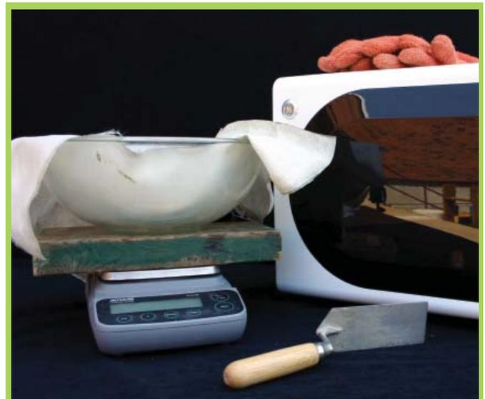
Figure 1. Microwave water content test equipment
