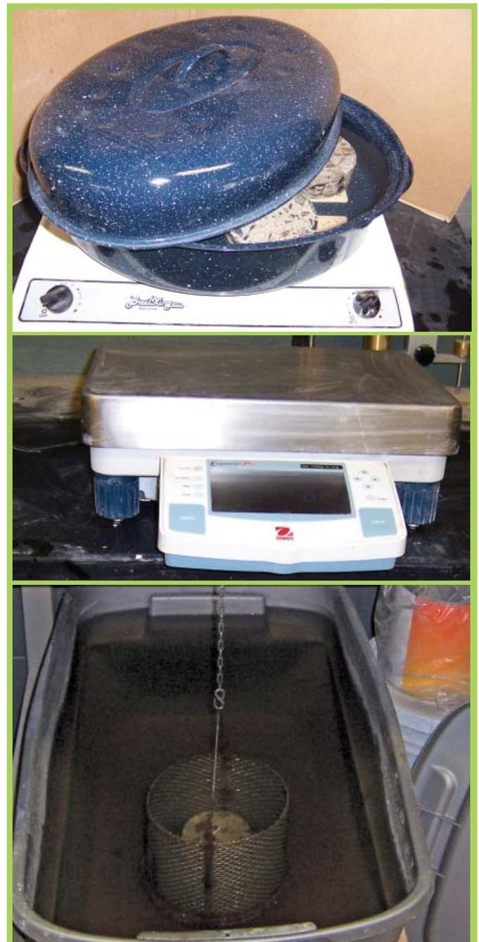
Figure 1. Boil test equipment
