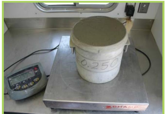
Figure 1. Unit weight test equipment
