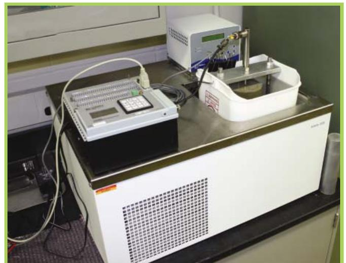
Figure 1. CTE testing equipment
