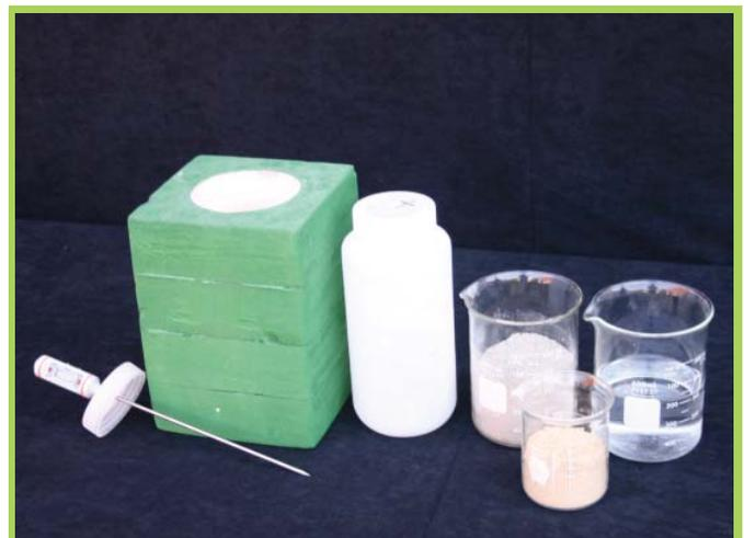
Figure 1. Cementitious heat generation test equipment and materials
