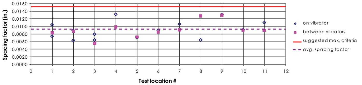
Figure 2. Spacing factor results (IA MCO demonstration project)
