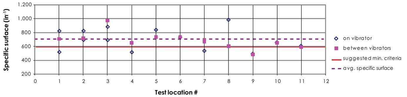
Figure 3. Specific surface results (IA MCO demonstration project)
