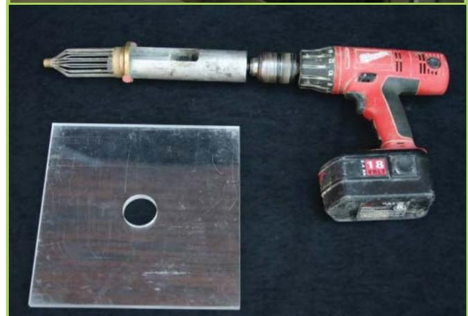
Figure 1. AVA setup in a portable lab and AVA sampling equipment
