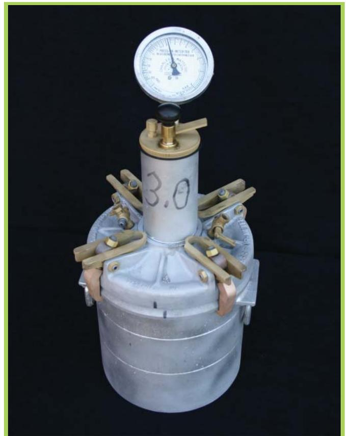
Figure 1. Air content test equipment (pressure meter)
