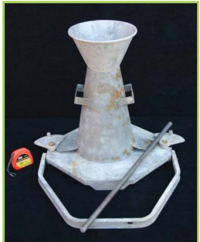
Figure 1. Slump testing equipment
